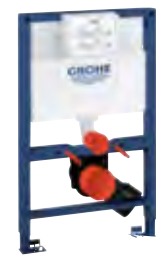
39 140 000 Rapid SL handicap for WC, flushing cistern GD 2 with small maintenance access 1.13 m installation height with fixing element for back support and bars, for WC bowls 70 cm projection
