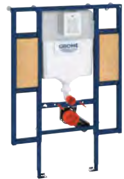
39 140 000 Rapid SL handicap for WC, flushing cistern GD 2 with small maintenance access 1.13 m installation height with fixing element for back support and bars, for WC bowls 70 cm projection
