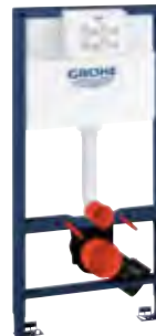
38 525 001 Rapid SL for WC with flushing cistern 3 – 6 l dual flush/start & stop/single flush, 1.00 m installation height connection from left/right/rear actuation from front/above
